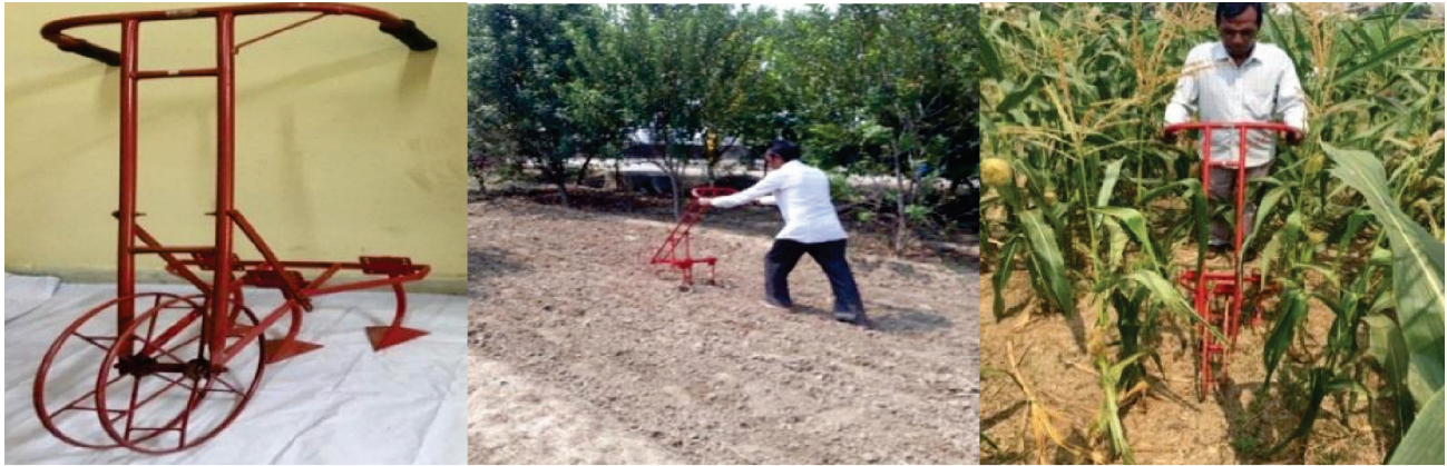
Plate 3. Evaluation of intercultural operation 3- row manual weeder
